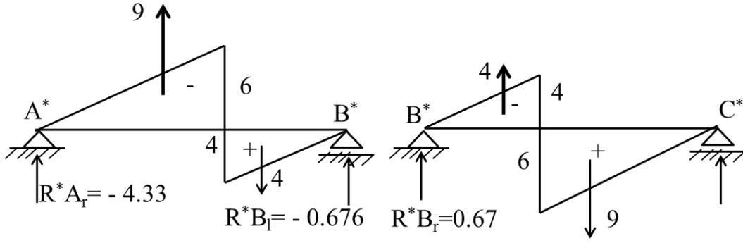
$$\Sigma MB^* = 0 \Rightarrow R_{Ar}^* \times 5 + 9 \times 3 - 1.33 \times 4 = 0$$
