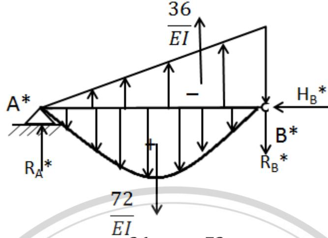
$$\Sigma MB^* = 0 \Rightarrow 6 RA^* + \frac{36}{EI} \times 2 - \frac{72}{EI} \times 3 = 0 \rightarrow RA^* = \frac{24}{EI}$$
