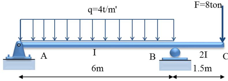
$$M_1 = 10x - 2x^2 \quad 6 \geq X_1 \geq 0 : \text{المجال AB}$$
